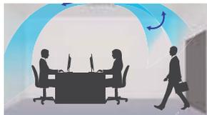
Individual louvers can be programmed separately. Adjust vertical airflow and louver position with UTY-RNRUZZ Wired Remote Control.
